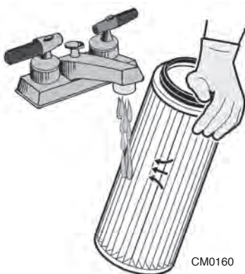
Wash the cartridge with tap water paying attention not to damage its cloth.
